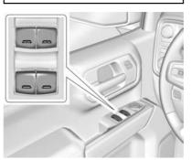
The power windows work when the ignition is on, in ACC/ACCESSORY, or when Retained Accessory Power (RAP) is active. See Retained Accessory Power (RAP)
