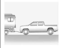
Only dinghy tow four-wheel-drive vehicles with a two-speed transfer case that have an N (Neutral) and a  $4 \downarrow$  (Four-Wheel Drive Low) setting.
