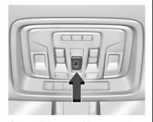
If equipped, the power sliding rear window works when the ignition has been turned on or to ACC/ACCESSORY, or Retained Accessory Power (RAP) must be active. See Retained Accessory Power (RAP) ⇒ 229.
