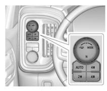
To activate Tow/Haul Mode turn the knob counterclockwise. To activate other drive modes turn the knob clockwise.
