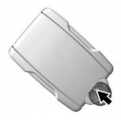
Separate and remove the back cover of the transmitter with a flat, thin object, such as a coin.
