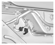
Replace the bulb and reverse Step 2 to reinstall.
