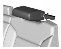
The head restraint can be folded forward to allow for better visibility when the rear seat is unoccupied. To fold the head restraint, press the button on the side of the head restraint.
