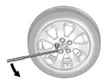
3. Use the wheel wrench and turn it counterclockwise to loosen the wheel nuts. Do not remove the wheel nuts yet.
