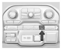
For vehicles without Driver Mode Control, press the Tow/Haul button on the center stack.
