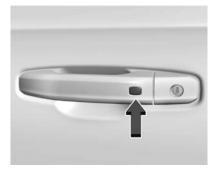
If equipped, the remote key must be within 1 m (3 ft) of the tailgate or door being opened or locked. Press the button on the door handle to open. See "Keyless Access Operation" in Remote Keyless Entry (RKE) System Operation (Key Access) ⇒ 10 or Remote Keyless Entry (RKE) System Operation (Keyless Access) ⇒ 13.
