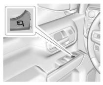
If equipped, press to power fold the mirrors. Press again to unfold.
