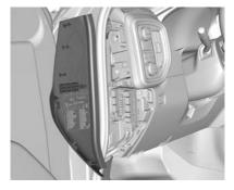
The left instrument panel fuse block access door is on the driver side edge of the instrument panel.
