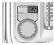
The cargo lamps provide more light in the cargo area or on the sides of the vehicle, if needed. The lamps inside the pickup box, in the tailgate handle, for the hitch, and/or the cargo mirror lamps also turn on, if equipped.
