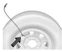
If equipped with a spare tire cable remove the cable from the spare tire by passing the clip through the looped end of the cable.
