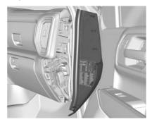
The right instrument panel fuse block access door is on the passenger side edge of the instrument panel.
