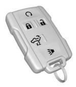
$\Omega$ : Press and release  $\widehat{\Box}$ , then immediately press and hold  $\Omega$  until the turn signal lamps flash or for at least four seconds. The engine may be started from outside the vehicle using the RKE transmitter. See Remote Vehicle Start  $\Rightarrow$  20.
