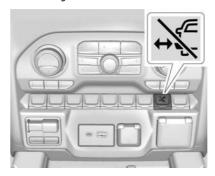
To extend both power assist steps for cleaning, press while the vehicle is in P (Park) or N (Neutral). Press again to retract them. The Driver Information Center (DIC) will display a message.
