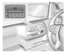
If equipped, memory seats allow two drivers to save and recall their unique seat positions for driving the vehicle, and a shared exit position for getting out of the vehicle. Other feature positions may also be saved, such as power mirrors, if equipped. Memory positions are linked to RKE transmitter 1 or 2 for automatic memory recalls.
