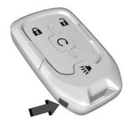
If the vehicle has the Keyless Access system, the transmitter has a button on the side of the transmitter used to remove the key.
