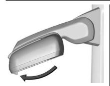
**Manual Extend:** If equipped, grasp the mirror housing firmly and pull back in one motion, arching slightly toward the rear of the vehicle.
