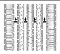
Treadwear indicators are one way to tell when it is time for new tires. Treadwear indicators appear when the tires have only 1.6 mm (1/16 in) or less of tread remaining. See *Tire Inspection* ⇔ 348 and *Tire Rotation* ⇔ 348 for additional information.
