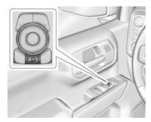
**Power Extend**: If equipped, press the power extend button to fully extend the mirror. Press again to retract.
