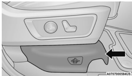
Pull Jack Access Cover From Front
